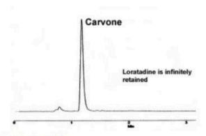
Chromatogram B Hexane 95% THF 5% Loratadine is Infinitely Retained
